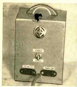
Rear view shows the ventilation cutout cover mounted above switch, S<sub>2</sub>. Another hole in the bottom of the box provides air circulation.
