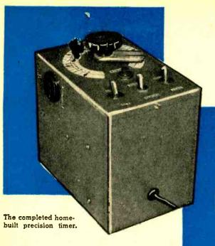
Accurate timing for enlarger or contact printer exposures up to sixty seconds.
