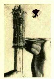
Electron gun, which later will be sealed into neck of a picture tube, receives final inspection after assembly. At bottom are leads and glass tubulation of stem assembly. Above, in order, are grid No. 1, grid No. 2, and metal sections of anode structure. At top is focus electrode, the "getter," etc.
