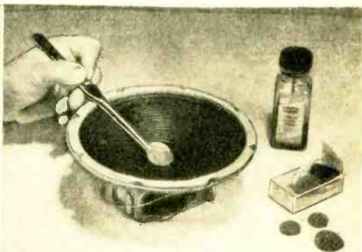
Fig. 8. Final step is replacing the felt pad over the speaker center by cementing it in place as shown. This pad keeps out dust.
