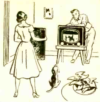
A picture with horizontal non-linearity. Note how the right-hand side of the picture is stretched out in contrast to left.
