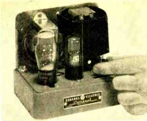
Fig. 4. General Electric's Model CR7505-K100 photo-relay unit with cover removed showing phototube, control tube, sensitivity control, transformer, and the relay.
