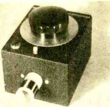
Fig. 3. "Nose"-end view of wavemeter with Coil A plugged in. Pilot lamp is at left.
