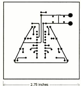
Fig. 2. This is the foil pattern for the Merry Christmas Tree. A kit that comes complete with a printed circuit board is available from Futurlec (see Parts List).
