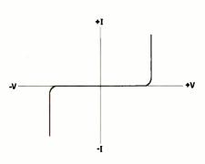
Fig. 2. A similar graph of two back-to-back zener diodes shows the difference in operation as compared to a diac, with the zeners having no upper-voltage trigger point.
