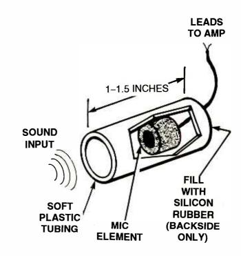
Fig. 1. The microphone element is housed in a 1- to  $1^{-1/2}$ -inch section of soft plastic tubing, with the area behind the microphone filled with silicon rubber
