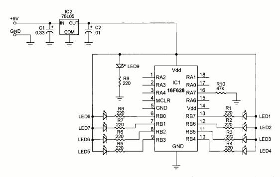
Fig. 4. The circuit isn't limited to a Christmas tree-or even LEDs. Using logic drivers and transistors, the output current can be upped to handle incandescent lamps and other devices-even a relay or solenoid.
