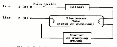
Wiring for Preheat Fluorescent Fixture using Automatic Starter
