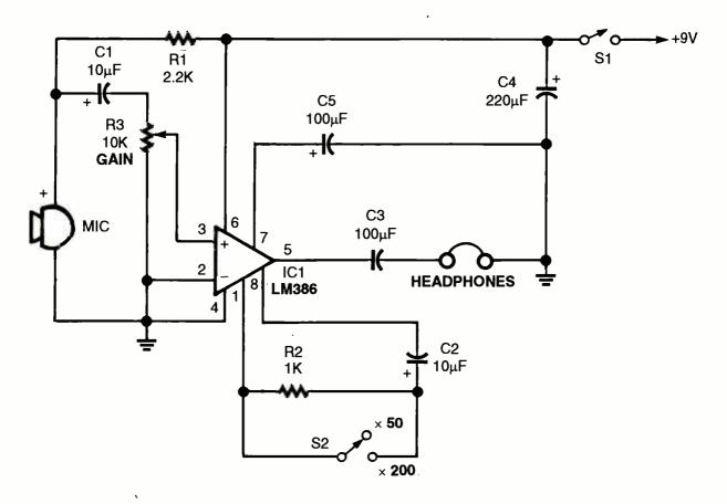
Fig. 2. The electret is connected to the amplifier circuit with a length of shielded microphone cable. If the microphone is to be used outside with the amplifier indoors, keep the cable length as short as possible.
