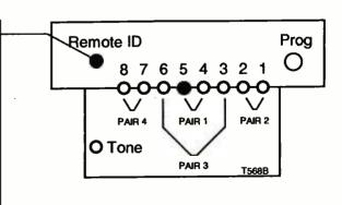
Fig. 5. With the remote unit in remote mode, identifying messages are sent down each wire to be received by a master unit.
