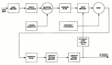
FIG. I. BLOCK DIAGRAM SSB TRANSMITTER USING FILTER METHOD
