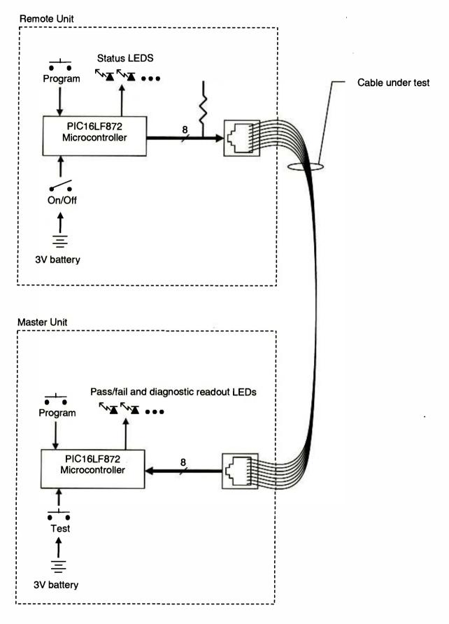
**36** Fig. 7. Block diagram of the Mapper8 master and remote units.
