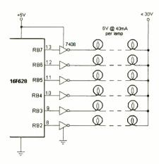
Fig. 1. The use of look-up tables greatly reduces hardware overhead, as seen in this schematic of flickering Christmas lights.
