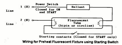
Fig. 2. The wiring for a preheat fluorescent fixture using a starting switch is different from that shown in Fig. 1.
