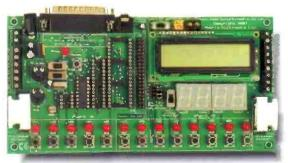
This flexible development board allows you to program 8, 18, 28, 40 pin PICmicro microcontrollers as well as test/develop code. All programming software is included and several resources which allow students to learn and program PICmicro microcontrollers are available - Flowcode, C for PICmicro microcontrollers and Assembly for PICmicro microcontrollers. A board is needed for the CD's below:
