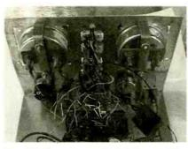
The variable power supply features two independent outputs, which are adjustable from 0 to 20 V<sub>DC</sub>. Two lead-acid batteries provide power; therefore, the device is completely portable.
