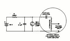
Fig. 3. A neon lamp relaxation oscillator was a favorite project for budding electronics hobbyists and could operate for nearly the shelf life of the battery.
