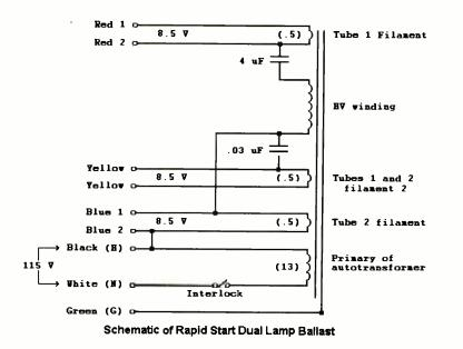
Fig. 7. This schematic shows the wiring for a rapid-start dual-lamp ballast.
