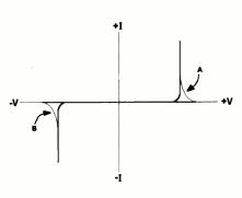
Fig. 1. This current vs. voltage graph of a diac is similar to that produced by a transistor curve tracer and shows the similarity of the device to a neon lamp.
