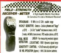
BROADBAND : 10 MHz to 4.5 GHz usable range HIGHLY SENSITIVE : Detects - Cellular phones and "Bugs" at 20 ft. - 2.4 GHz "sealed" microwave ovens at 40 ft. 2 meter, 440 MHz transceivers, FRS walkie talkies at 80 ft. DUAL MODE : LINEAR · For measuring weakest signals DETECTION : LOGARITHINC - 1000:1 dynamic signal range SENSITIVITY CONTROL : > 20 dB manually adjusted pain
