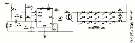
Fig. 5. A strip of 15 LEDs under the stationary cutting edge of a paper knife will cast a shadow, allowing precise paper positioning against the edge. A 555 timer allows the strip of LEDs to stay on for 30-second intervals for operators who forget to turn the light source off.
