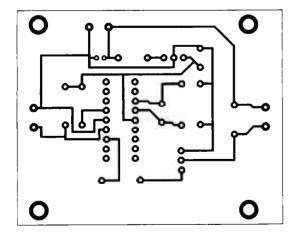
Fig. 2. This PC-board foil pattern can be utilized to etch your own boards. An etched and drilled board is available from the P C author for a nominal charge, as is a pre-programmed PIC chip.
