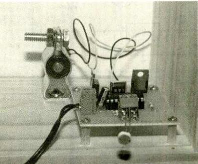
Simulate the clip-clop of Santa's sleigh team on your rooftop. turns on transistor Q1, which controls the solenoid. The solenoid is mounted inside a wooden box, giving a nice, resonant "clop, clop" sound when its piston strikes the side of the box.
