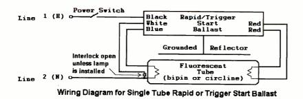
Fig. 3.Here's the wiring diagram for the single-tube rapid- or trigger-start ballast.
