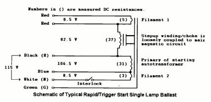
Fig. 5. This schematic of a typical rapid/trigger-start single-lamp ballast is shown here.
