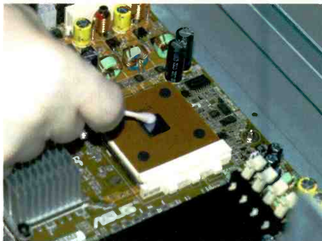
Photo 3. Take extra care in cleaning the contact point of the CPU that will bond with the heatsink. Here a cotton swab is dipped in rubbing alcohol and swabbed over the CPU's center.
