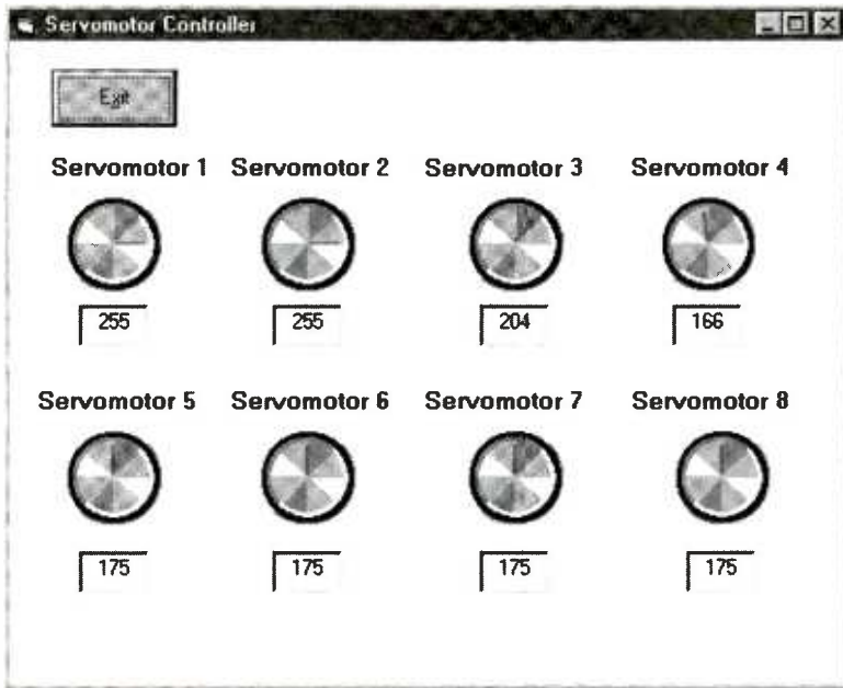
The Visual Basic program I wrote has been tested under Win95 and Win 98. The program continually updates each servomotor position, but not as quickly as needed for completely smooth operation.
