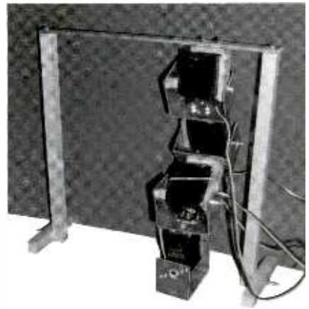
While this stand works, it is a little small (short) for the application. At times the leg can lift and topple itself along with the stand. It appears possible that when both servo motor legs are attached they will be able to lift and walk the stand in place.
