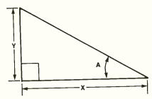
Fig. 5. Arctangent is the angle (A) that corresponds to the ratio of the length (Y) divided by the length (X).
