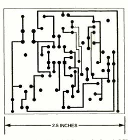
Fig. 8. Here is the solder-side foil pattern for the main PCB
