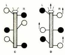
Fig. 1. The above diagram shows the tripod gait of a hexapod. There are always three feet on the ground at any given time.
