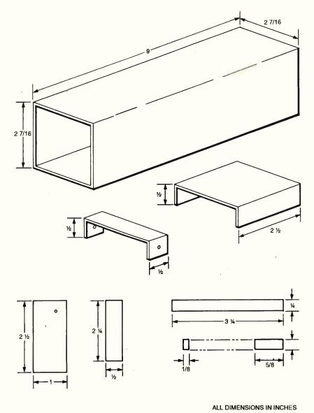
Fig. 1. The Electronic Mouse Trap consists of a rectangular corridor with a spring-loaded door at each end. An LED/photodetector circuit acts as a trigger. The dimensions for each plastic piece are given above.
