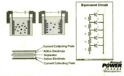
An ultracapacitor consists of two non-reactive porous collecting plates suspended within an active electrolyte. When a voltage is applied across the plates, the positive plate attracts the negative ions in the electrolyte, while the potential on the negative plate attracts the positive ions. This effectively creates two layers of capacitive storage.
