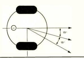
Fig. 3. Mechanical differences in the motors' speed can cause the robot to go at undesired angles.
