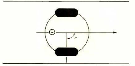
Fig. 2. When the robot is parallel to the wall, the angle of correction is 0. That angle does not affect the speed of either wheel, resulting in the robot traveling straight down the hall.
