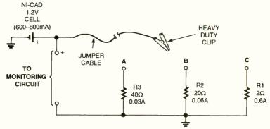
Fig. 1. This is a simple circuit for monitoring and testing the capacity of NiCad AA cells. The only components needed are inexpensive resistors.
