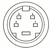
Fig. 1. The S-Video plug as viewed from the "solder tab" end, illustrating the pin locations as described in the text, is a 4-pin "mini-DIN" type of connector.
