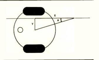
Fig. 4. When the robot is not in the middle, a second angle of correction can be calculated.
