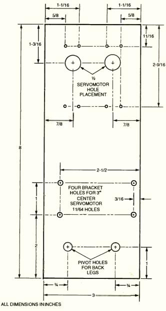
Fig. 3. The above figure can be used as a template for constructing the hexapod's body.
