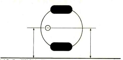
Fig. 6. Two Sharp GP2D12 Infrared Distance Sensors are mounted on the robot facing the same wall.
