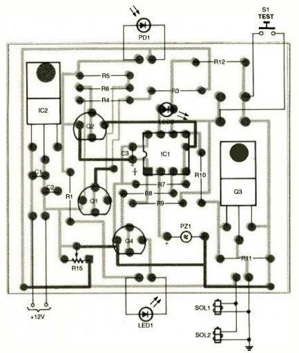
Fig. 6. Use the parts placement diagram above as a reference for constructing the Electronic Mouse Trap. Make sure to observe capacitor polarity.
