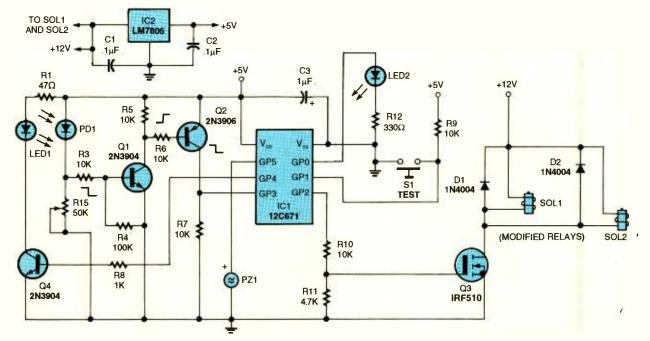
Fig. 4. The schematic above shows the circuit for the Electronic Mouse Trap. The circuit is controlled by a PIC12C761 microcontroller. Note the locations of LED1 and PD1. When an object 32 blocks LED1's light from hitting PD1, the solenoids activate and release the doors.
