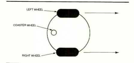
Fig 1. When both wheels are turning at the same speed, the robot travels straight down the hall.
