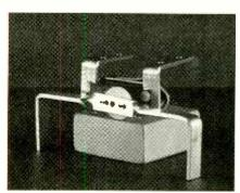
The center servo is shown here ready to be attached to the body. The center legs and the two L-brackets have been attached to the servo.
