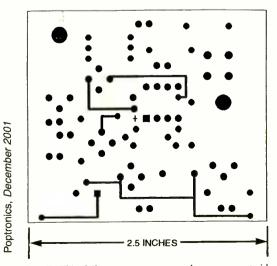
Fig. 7. This foil pattern represents the component-side 34 copper trace.
