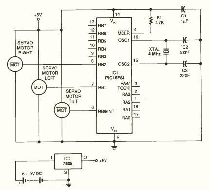
Fig. 8. At the heart of this hexapod lies a PIC16F84 with an external 4-MHz crystal linked to the oscillator pin-outs, 16 and 15.
