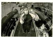
This shield protects the giant Z-Beamlet's final focusing lens from debris when the Z accelerator fires. The lens is square because the beam generates a footprint that's about one square foot, which is then focused down to about 100 microns.
