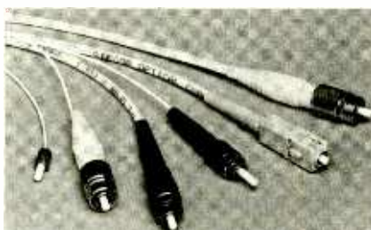
Fiber-optic cable comes in many varieties as seen above. Drastic measures are taken to protect fragile glass fiber. An outer layer of PVC combines with a mesh tube of Kevlar surrounding the fiber to form a shield. The tips of the cable are then spliced to special connectors that allow the cables to be plugged into various transceivers and multiplexing equipment.
