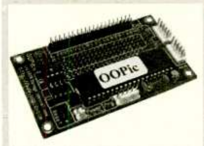
The OOPic II has a large number of robotic sensor software objects, including one that reads the Sharp GP2D12.
