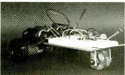
Here is a Braitenberg Vehicle ready to go. The batteries are docked at the rear.
