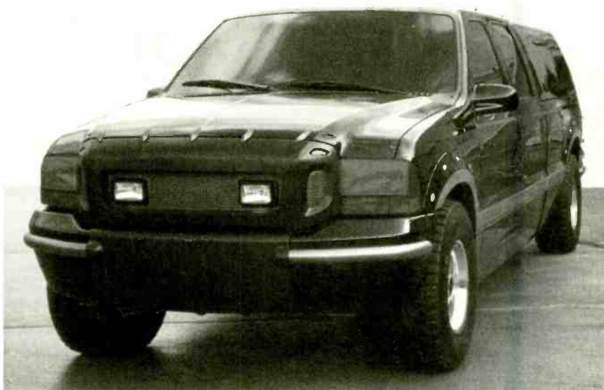
Army designers used the Ford F350 heavy-duty pickup truck to develop the military's latest SmarTruck.
