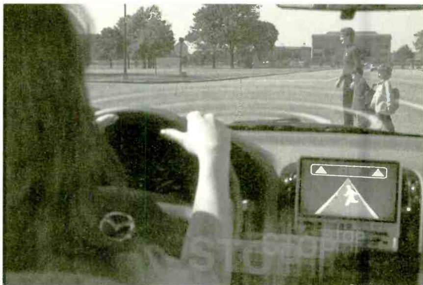
SensorCar's forward-looking radar can recognize pedestrians and working with a computer can determine if they are in danger.
