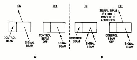
Fig. 2. There are two main types of optical switches: transmissive (A) and reflective (B). Both of them can keep a beam from traveling to a particular destination, but a reflective switch can redirect the beam to a new destination.
