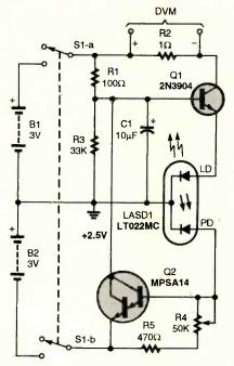
Fig. 5. Note the simplicity of the driver circuit used for the LT022MC 780-nm, 5-mW doubleheterostructure laser diode. The ±3-volt supply is merely four "N" cells
