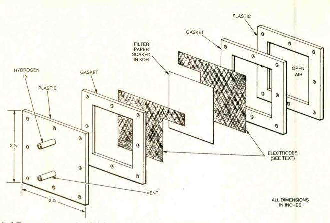
Fig. 2. The construction cross section of the hydrogenloxygen fuel cell is a sandwich of electrodes, electrolyte-soaked paper, and gaskets surrounded by a pair of flat plastic end pieces.
