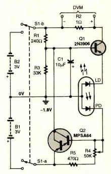
Fig. 6. Due to its common-anode package configuration, the ML720 1300-nm, 5-mW DH laser diode uses a "flip-flopped" version of the driver shown in Fig. 3.
