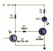
Fig. 3. This detector circuit uses a second transistor to drive an LED indicator.
