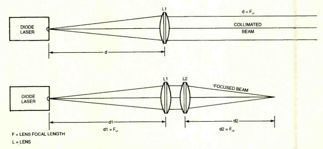
Fig. 4. Collimating and focusing a semiconductor laser takes a bit more thought than the He-Ne variety. Compare this illustration to that in Fig. 2 for the differences. Note that you have to work with a more diverging beam with semiconductors.
