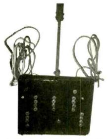
It's a black box. It's a VCR. It belongs to ET. No, it's KOOL CHEK, an automotive tester that pinpoints malfunctions in the cooling system of a liquid-cooled internal-combustion engine—especially in the engine's thermostat.
