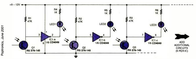
Fig. 5. Although only three stages of the Fig. 4 circuit are shown, you can have six detectors per IC **58** chip—one for each gate.
