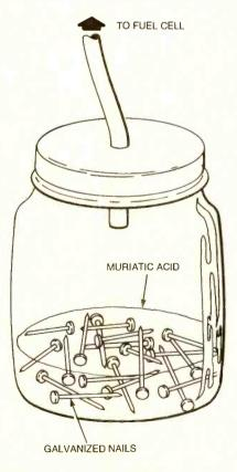
the hole. Make the junction between the jar lid and tube airtight by coating the seam—both on the top and bottom of the lid—with aquarium silicone sealant. Allow the sealant to dry (about 24 hours).
