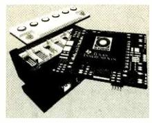
Seen here is a cross section of the iQ Power smart battery. The "brains" of the system are microcontrollers from Texas Instruments.
