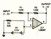
Fig. 5. This reader-designed unity gain op-amp inverter is intended to reverse the output "phasing" of an automotive sensor.
