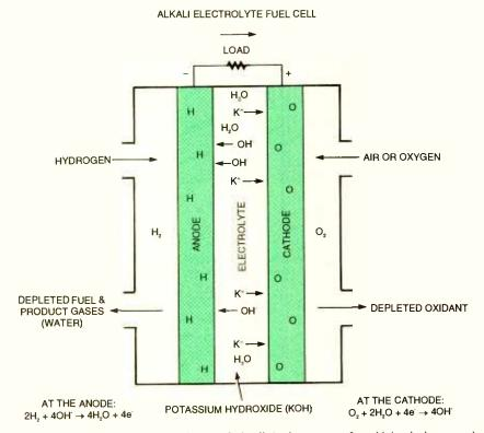
Fig. 1. An alkali-electrolyte hydrogen/oxygen fuel cell, in the process of combining hydrogen and oxygen, strips a few extra electrons during the chemical reaction to create an electromotive forceelectricity.
