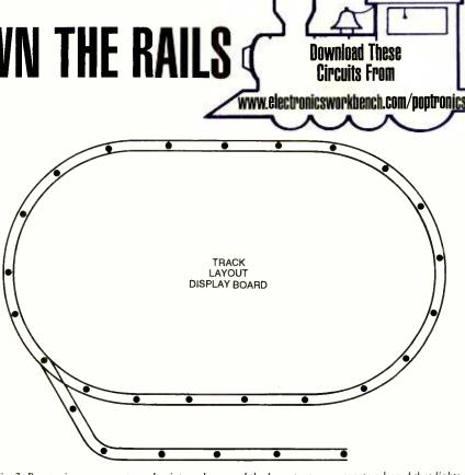
Fig. 2. By spacing sensors at regular intervals around the layout, you can create a board that lights up to indicate train position.
