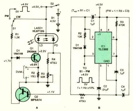
Fig. 7. The 670-nm, 5-mW visible DH laser driver (A) uses only a positive supply and may be operated in either continuous or pulsed mode. The simple fixed oscillator shown (B) provides a 50-ms pulse at a 2-Hz rate.
