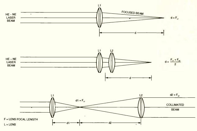
Fig. 2. Collimation and focusing of laser beam emission is quite easily accomplished using short focus (over ½ inch) small diameter glass or plastic lenses. If you require shorter focal lengths, stack two similar lenses back to back—the effective focal-length is then halved.
