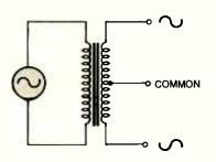
Fig. 2. The traditional phase splitter "divides" the original signal into two complementary signals using a unity-gain amplifier.
