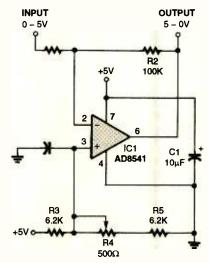
Fig. 6. Modifications to the unity-gain op-amp inverter include a "rail-to-rail" op-amp and additional offset adjustment circuitry.
