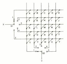
Fig. 1. A simple set of rotary switches makes it easy to select a particular intersection in a matrix.
