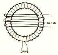
Fig. 1. In a fluxgate sensor, a donut-shaped core is pulsed with a field to saturate it. When the field collapses, the sense windings generate a current based on how much an external magnetic field rushes in to fill the void created by the collapsing drive field.
