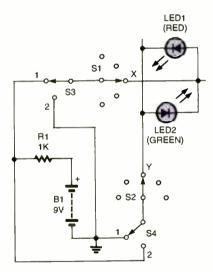
Fig. 3. By adding an additional pair of switches, you can reverse the current polarity, lighting a second LED.
