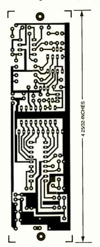
Fig. 8. The Fluxgate Magnetometer circuit fits neatly on a single-sided PC board.
