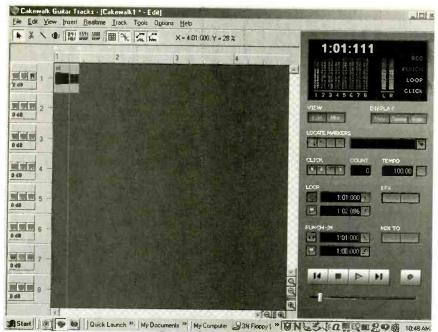
Here is screenshot of the Special Information Tone as seen in Cakewalk's "Guitar Tracks" soundeditor. The tones are descending in volume, but ascending in frequency. The tones are: 985.2 Hz, 1370.6 Hz, and 1776.7 Hz.
