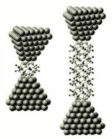
The simulations also suggest a way that could overcome some of the anticipated problems involved in doping the silicon used in devices this small. Because the clusters form hollow cages, much like carbon fullerenes, they could be fabricated around a dopant atom. With each cluster then containing a dopant atom, device consistency may be achieved.
