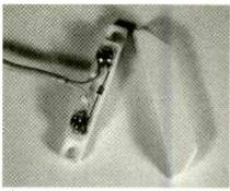
The reed switch at the mailbox has convenient solder tabs for connecting D3 where it's needed most—to protect the reed switch.
