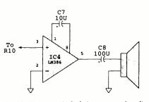
Fig. 10. If you can't find the suggested audio amplifier IC, you can substitute an LM386 cheaper and widely available.
