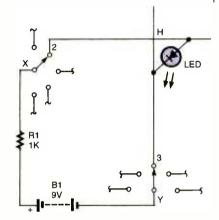
Fig. 2. The switches from Fig. 1 can power an LED connected at the matrix cross-over points.
