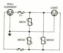
Fig. 2. A surge protector using voltage-clamping metal-oxide varistors (MOVs) will react quickly and reliably, protecting the load from damaging transients.
