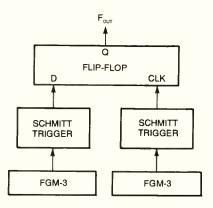
Fig. 4. A digital mixer takes the outputs of two fluxgate sensors and combines them into a difference signal.
