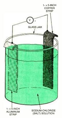
Fig. 1. An aluminum battery is a simple variation of the more familiar lead-acid "wet cell" battery found in cars.
