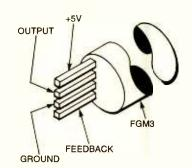
Fig. 3. The FGM-3 has four pins for connecting to an outside circuit.
