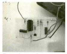
The circuit fits on a small piece of perfboard. Cut to the right size, the board can fit in the retention slots of an experimenter's project box.
