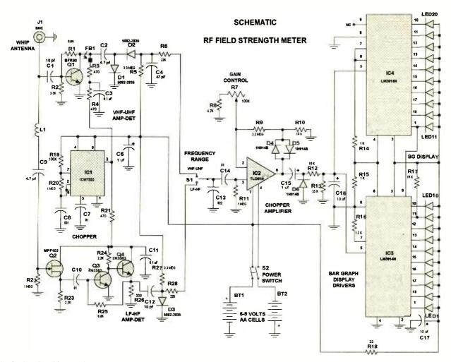
Fig. 2. The RF Field-Strength Meter is a simple detector that is amplified to the required sensitivity without being over-sensitive to the point of being useless.
