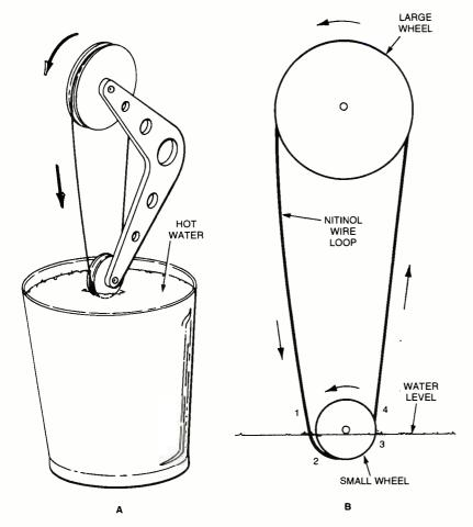
Fig. 4. Detail and function of the Nitinol loop used to power the Thermobile.
