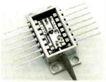
Alignment structures, less than a 10<sup>th</sup> of an inch in size in this optical module, use the LIGA microfabrication process. This AXSUN Technologies photonic subsystem sits on an electronic assembly that occupies about 60 percent of the area of a business card (2.5 inches long by 1.7 inches wide).
