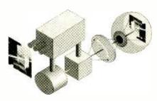
Fig. 1. The Microvision Virtual-Retinal Display consists of four main parts to translate the source image from a computer or camera into an image projected on the eye's retina: drive electronics, a modulated light source, horizontal and vertical scanners, and viewing optics.
