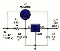
Fig. 2. This circuit lets an LM7812 pass four amps or more. Both the transistor and the voltage regulator will require good heatsinks. The same trick will work with any three-terminal regulator of the 78xx series.
