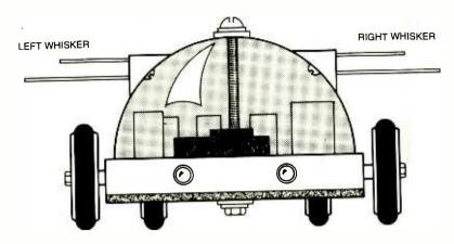
Fig. 4. "Whiskers" added to a robot give it a "cat-like" ability to sense when something is close without having to ram into the object.
