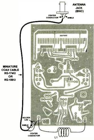
L1 = 4 TURNS #22 WIRE 1/4" DIA, 1/2" LONG NOT CRITICAL AS TO EXACT INDUCTANCE BARE OR INSULATED WIRE USABLE
