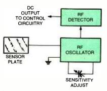
Fig. 1. One simple form of proximity sensor relies on body capacitance. Radio-frequency (RF) oscillators are sensitive to stray capacitance due to the extreme frequencies they generate. A simple detector for the frequency shift can control any electrical device. That sensitivity is why you should use insulated tools when adjusting tuned circuits in radios and TVs.
