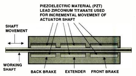
Fig. 3. In the same way that standard electric motors have been "opened out" flat to form linearinduction motors, ultrasonic motors can also work in a linear fashion. This so-called "inchworm" motor uses two "brakes" that surround a central "extender," Ultra-precise movement-in the nanometer range—is possible with this arrangement.
