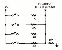
Fig. 6. A resistor ladder provides a way to tap multiple voltage levels. The voltage at the output of the ladder is dependent on the switch(es) that
