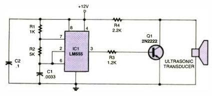
Fig. 1. Schematic diagram for a basic ultrasonic proximity transmitter.
