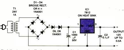
Fig. 1. Here is a complete 12-volt power supply using a 24-volt transformer. See the text for we explanation and suggested improvements.
