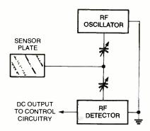
Fig. 5. A subtle yet substantial variation on the Fig. 1 concept is to detect a change in an RF signal after it has left the oscillator; in Fig. 1, the oscillator is directly affected by the sensor plate.
