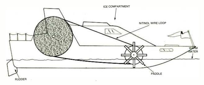
Fig. 6. This cross-section of the Cool-Craft shows the Nitinol loop and the bottom paddle.
