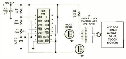
Fig. 3. This inverter circuit will run a 60-Hz electric-clock motor from a 12-volt DC source. Adjust R1 for a 60-Hz frequency.
