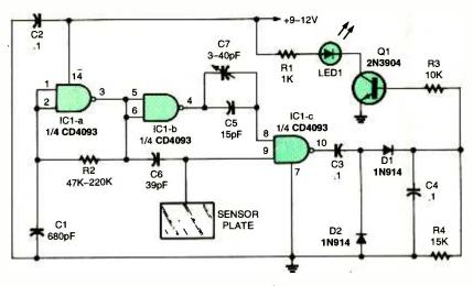
Fig. 4. The simplest way to detect phase changes is with digital-logic gates.
