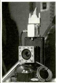
Infrared Ranging via Image Subtraction (IRIS) sensors can see through fog. IRIS capitalizes on the fact that all vehicles contain retroreflective surfaces. On automobiles, these are found in taillights. IRIS captures and compares two images: one illuminated with its infrared beam and the other illuminated by ambient light. The difference between the two images is the retroreflective surface, enabling you to see taillights or a reflective bumper sticker. (Photo by Todd Cheney, UCLA.)
