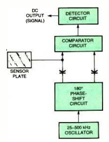
Fig. 3. Another technique is to compare two identical signals that are 180° out of phase. If one signal shifts in phase, the comparator detects the difference and outputs a signal.
