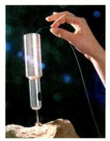
This drill, developed at NASA's Jet Propulsion Laboratory, weighs about a pound but can drill with a jackhammer-like motion through rock as hard as granite or basalt. The broken debris is drawn up through the hollow drill shaft. The resulting hole is little bigger than the drill head.
