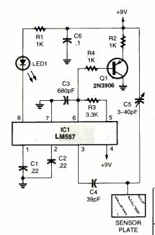
Fig. 6. Although the LM567 is designed to not have interference between its internal oscillator and detector, we've tricked the chip to do just that.
