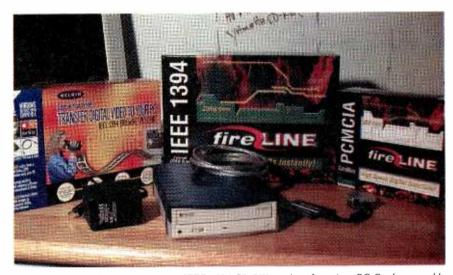
The Evergreen Technologies fireLINE IEEE-1394 CD-RW can interface via a PC Card or an addin PCI card like this one from Belkin.
