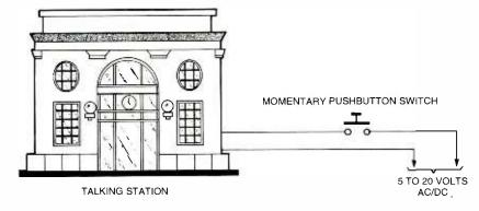
Fig. 2. How to set up the Talking Station circuit for manual operation.
