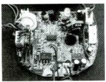
The main PC board contains most of the electronic circuitry. The position sensor is at the upper left corner, while two daughter boards (each with a custom microporcessor) are located at the left.
