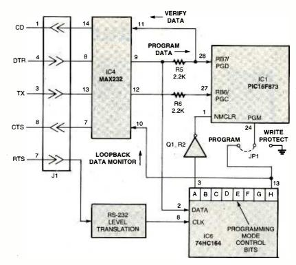
Fig. 2. This detail shows the PIC-programming portion of the GameEnhancer.
