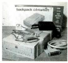
The Backpack CD-rewriter drive from Micro Solutions is an external drive that can connect to your PC or laptop using a parallel-port cable or through a USB interface.
