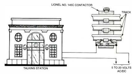
Fig. 3. How to set up the Talking Station for automatic operation.
