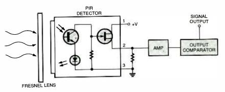
Fig. 3. Most PIR sensors are large, transistor-like devices with a somewhat common pinout arrangement, like the one shown here.
