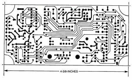
Fig. 5. Here's the foil pattern for the solder side of the GameEnhancer. Note that the board was designed so that soldering components on the component side is not required; only the via holes carry signals between the two sides.
