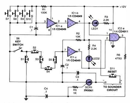
Fig. 1. This alarm circuit can handle both normally open and normally closed sensor switches. All you need to add is a suitable power supply and a siren.
