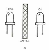
Fig. 1. The basic design of the infrared proximity sensor.
