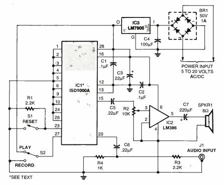
Fig. 1. The full schematic of the Talking Station.
