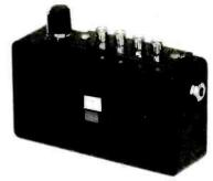
Fig. 7. Several holes need to be located and drilled for mounting the external components of the GameEnhancer. Note the rectangular hole for DISP1 and the "speaker-grille" hole pattern.
