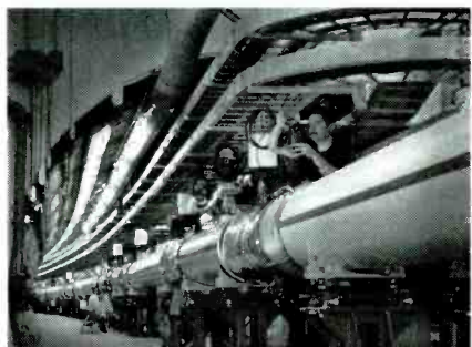
A view of the superconducting magnets at RHIC. As gold particles zip along the collider's 2.4-mile-long tunnel at nearly the speed of light, 1740 of these magnets guide and focus the particle beams.
