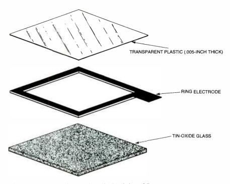
Fig. 3. The ring electrode is not hard to make. Just do it carefully.
