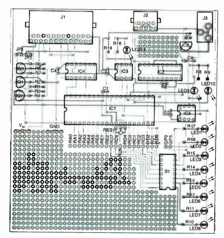
Fig. 5. When building the IAPDB, use sockets for the ICs. Don't forget to make connections on both sides of the board.
