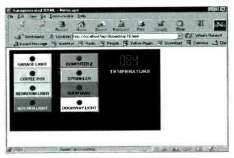
Fig. 18. Accessing the embedded HTML code in the IAPDB demonstration software shows how you can read information (temperature) as well as issue commands. If you replace the LEDs on the IAPDB with transistors or solid-state relays, you could control the displayed devices by clicking on them. With the IAPDB connected to the Internet on a permanent basis, you could do that from anywhere in the world!
