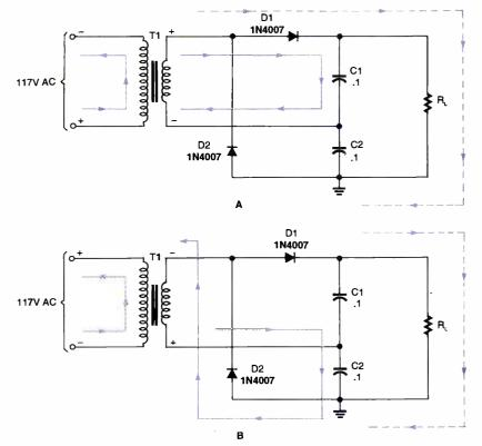
Fig. 3. For the sake of greater clarity, the full-wave voltage doubler illustrated in Fig. 2C can be redrawn as shown here. The full-wave voltage-doubler circuit has better regulation, is easier to filter, and produces nearly double the peak AC voltage of the half-wave version.
