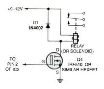
Fig. 4. For heavy-duty requirements over 100 mA, a hexFET driver is needed to handle the higher current load.
