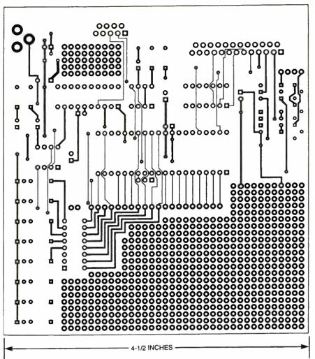
A Data Link Module, or DLM. Fig. 4. Here's the foil pattern for the solder side. Note that large amount of space for prototyping additional circuitry.
