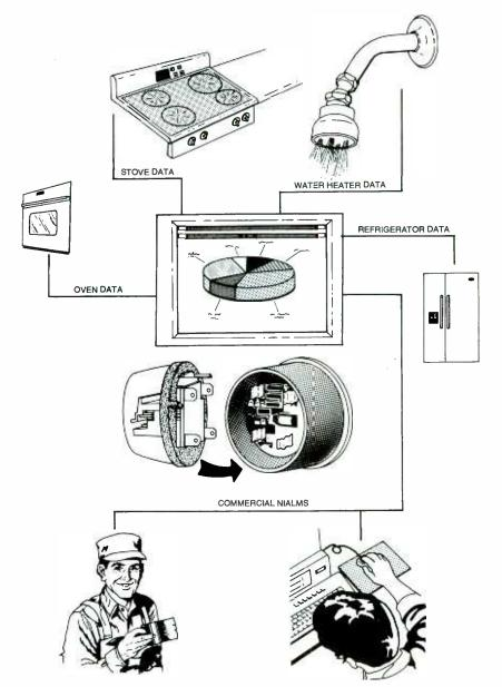
Fig. 1. The NIALMS Field Recorder is installed on the home's utility meter in between the meter box and the meter, as shown here.
