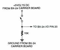
Fig. 1. Wire the switch so that it connects to the V+ (pin 21, not pin 24) of the BX-24.
