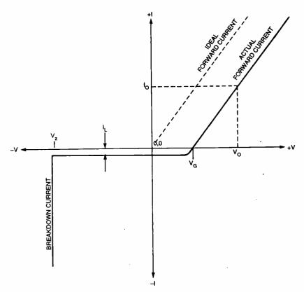
Fig. 2. The transfer characteristic of a practical (non-ideal) solid-state diode is shown here. Unlike the ideal diode, there is a minute leakage current (IL) flowing backwards across the junction in a practical diode.
