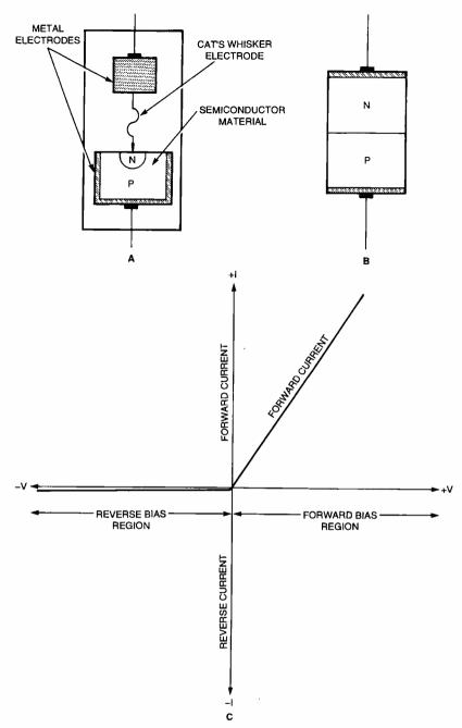
Fig. 1. Solid-state diodes are available in two different configurations; point-contact (A) and junction (B) types. The current-vs.-voltage characteristic of the "ideal" PN-junction diode is illustrated in C. Note that there is no reverse-current flow through an ideal diode when reverse biased.
