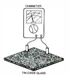
Fig. 2. When you find the conductive side of the glass, the ohmmeter will read a low resistance.
