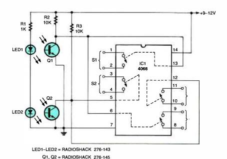
Fig. 1. This simple electronic switch is built around two pairs of infrared LEDs and phototransistors. The CMOS analog switches isolate the phototransistors from whatever load you want to drive.
