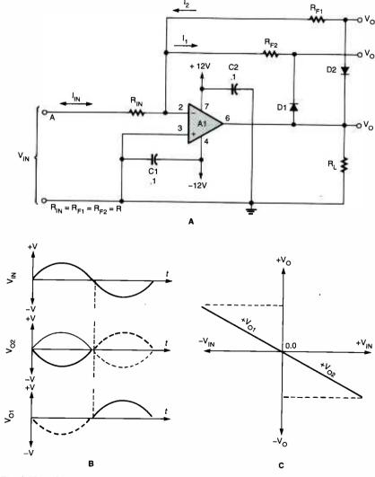
Fig. 6. The polarity discriminator shown in A—a circuit built around the inverting voltage-follow-er—indicates whether the input voltage is zero, positive, or negative. The circuit's input and two output waveforms are shown in B, and the circuit's transfer characteristics are shown in C.
