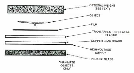
Fig. 1. Everything is set up for taking a Kirlian photo. In some instances, you might want to place a sheet of clear glass over the object being photographed.
