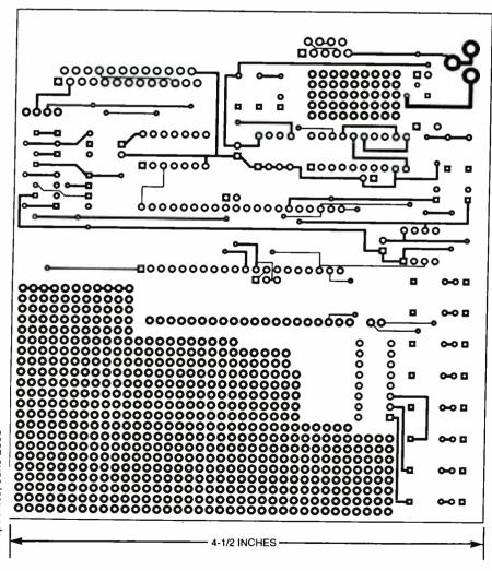
30 Fig. 3. The IAPDB uses a double-sided board; here's the foil pattern for the component side.
