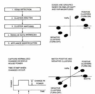
Fig. 3. By analyzing the raw data captured by the recorder, NIALMS can recognize individual appliances by their usage pattern.
