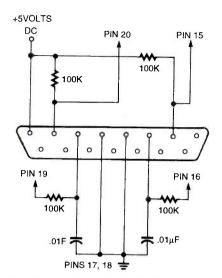
Fig. 2. Connecting an IBM PC-style joystick to the BasicX-24 microcontroller.
