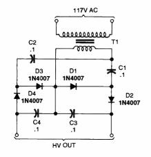
Fig. 5. Like the voltage tripler, this circuit (a voltage quadrupler) is based on the voltage-doubler of Fig. 3 and operates in much the same manner.
