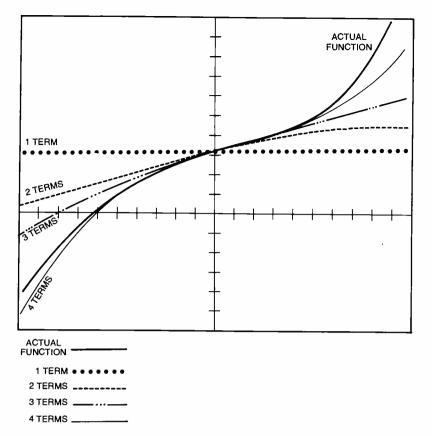
Fig. 2. Taylor Series deals with nonlinearity by breaking a curve down into separate terms.
