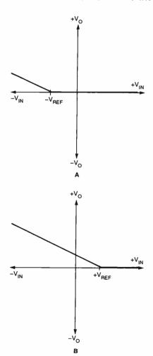
Fig. 10. The transfer characteristics for the circuit in Fig. 9 are shown here. In A, V<sub>REF</sub> is negative, while V<sub>REF</sub> is positive in B. In both cases, the transfer curve is offset by the reference signal.
