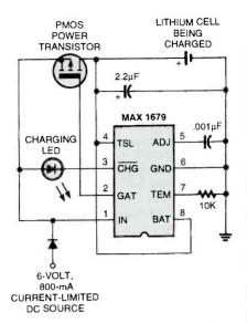
Fig. 4. Special charging circuits are needed to safely charge lithium cells. This example uses a new Maxim chip.
