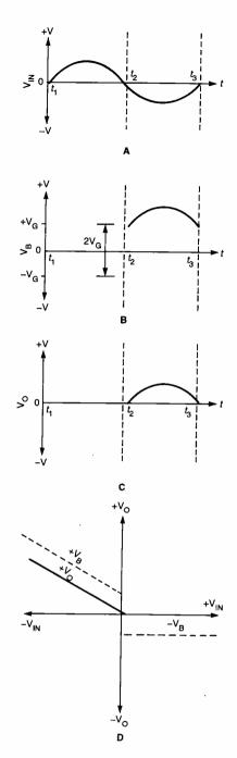
Fig. 4. These waveforms help to illustrate the operation of the precise rectifier. The illustration in A shows the input waveform, B shows the waveform at the output of the op-amp, C shows the circuit's output waveform, and D shows the same situation graphically.
