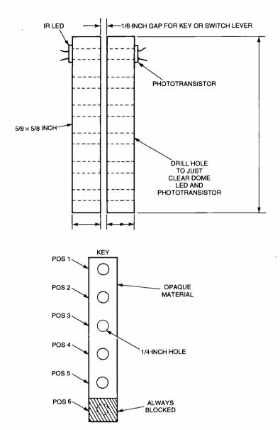
Fig. 6. One way you can arrange the IR LEDs and phototransistors is to create a slot for the key. As you swipe an opaque card with holes cut in it to match the required pattern of blocked and unblocked pairs, the circuit activates when the patterns match.
