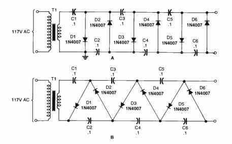
Fig. 6. Note that the circuit in A is electrically identical to the one in B. The usefulness of these circuits can be enhanced by adding voltage taps at each of the diode junctions (D1/D2, D2/D3, D3/D4, D4/D5, and D5/D6) to provide for multiplication factors of  $\times 1$ ,  $\times 2$ ,  $\times 3$ ,  $\times 4$ , and  $\times 5$ .
