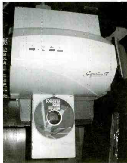
Fig. 4. The finished CD-R disc emerges from the Primera Signature III CD Printer.
