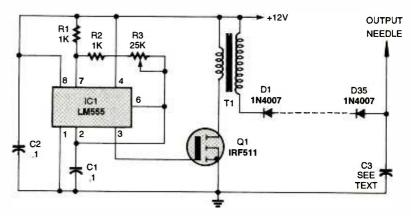
Fig. 6. A solid-state circuit is the most versatile method of building a negative-ion generator. By adjusting the frequency of ICI with R3, you can tune the circuit to the resonance of TI for greatest efficiency. Any 12-volt automobile ignition coil will do for TI.
