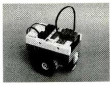
Fig. 2. Here's the basic rover robot equipped for the sample NQC program in Listing 1. It's equipped with two drive motors and a light sensor.
