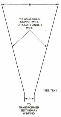
Fig. 2. A Jacob's Ladder is simply a pair of solid wires that form a "V" shape. When a spark jumps the narrow gap at the bottom of the device, it ionizes the air, creating a low-resistance path. The heat generated by the spark causes the air around it to rise, carrying it up the ladder. At the top, the spark breaks off. At that point, the path of least resistance for the current returns to the narrow gap at the bottom, and the show repeats.
