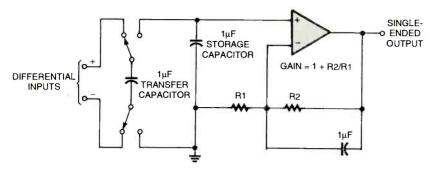
Fig. 3. This amazingly versatile capacitor-switching scheme offers unusual circuit possibilities.
