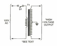
Fig. 1. Neon-sign transformers are good sources of high voltage for experimentation. Several safety features are usually built into these devices. For example, the center tap is usually connected to the circuit's case-a good ground for eliminating potential shock hazards.
