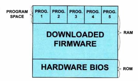
Fig. 1. The Mindstorms RCX uses a hardware BIOS in ROM, along with firmware and program data in RAM. Note how only five programs can be stored at a time.
