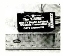
Fig. 4. A higher-powered video transmitter such as the Ramsey unit pictured here can send signals a far as <sup>1</sup>/2 mile. Check your local regulations concerning the maximum power allowed for unlicensed transmitters. Note that this unit transmits on Cable Channel 59; you'll need a television that can pick up that frequency as it is not within the standard broadcast frequencies.
