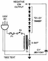
Fig. 3. Rectifying the high-voltage output of a tapless high-voltage transformer makes a simple negative-ion generator. It's a good idea to use four times as many diodes as their breakdown voltage indicates as a safety factor against one diode failing.
