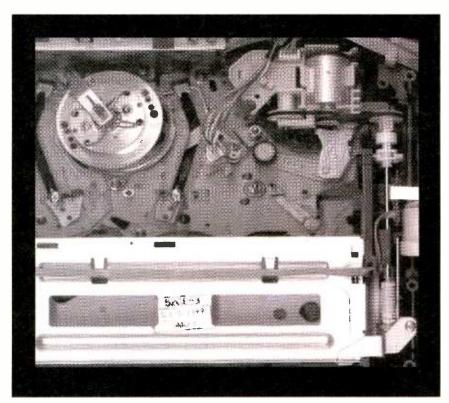
Fig. 1. A typical VHS VCR tape transport mechanism.
