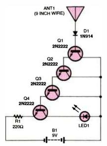
Fig. 1. While this circuit might seem to be a serviceable field-strength indicator, its floating input will pick up everything from passing cars and people to what might be interpreted as "other-worldly spirits!"
