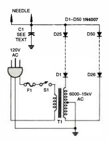
Fig. 5. If you'd like to build a negative-ion generator but can't find a tapless transformer, this circuit will fill your needs. Note that two strings of diodes are used instead of the single string shown in Fig. 3.
