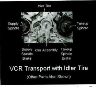
Fig. 2. This VCR mechanism uses an idler tire instead of gears. (Photo courtesy of Brian Siler.)
