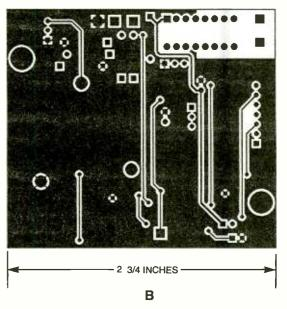
Fig. 4. The Electronic Padlock was assembled on a double-sided printed-circuit board, measuring 2 3/4 × 2 1/2 inches. Full-size templates of both sides of the unit's dual-pattern layout is shown here. The component side is shown in A, while the bottom layer is
