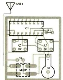
Fig. 4. The transmitter, thanks to its low parts count, is small and compact. Note that MOD1 is installed on the solder side of the board.
