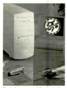
Try locking up your PC with the Data Defender—it's as easy to use as the key that opens your front door. When it's not in your system's parallel port, the machine won't boot.
