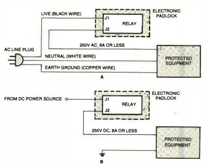
Fig. 2. The load's power source (AC or DC) dictates the manner in which the load is connected to the Electronic Padlock. The diagram in A illustrates how AC loads can be safely connected to the Padlock, while illustration B outlines DC-load connection.
