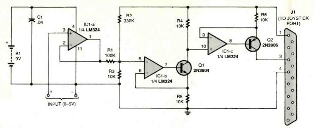
Fig. 2. This circuit will let you use a PC joystick port as a voltmeter in conjunction with the program given in Listing 1.
