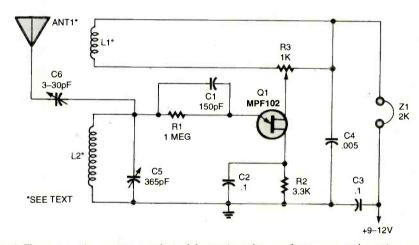
Fig. 6. The regenerative receiver, popularized during the radio era of yesteryear, replaces the vacuum tube used in the original design with an MPF102 JFET.
