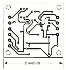
Fig. 2. Here's the foil pattern for the Caller-ID Alarm.
