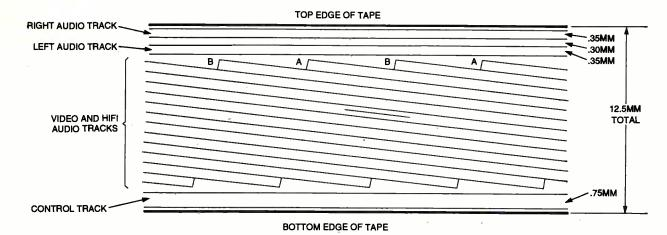
Fig. 2. Each track on a VHS tape corresponds to one field of the interlaced video format. One rotation of the drum corresponds to a complete video frame with the heads designated A and B for the even and odd fields, respectively.
