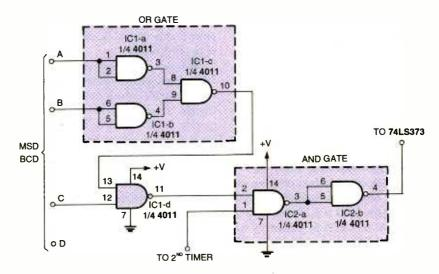
Fig. 1. The error-code detector (ECD) is comprised of OR and AND gates manufactured from common 4011 CMOS NAND gate chips, as shown here.
