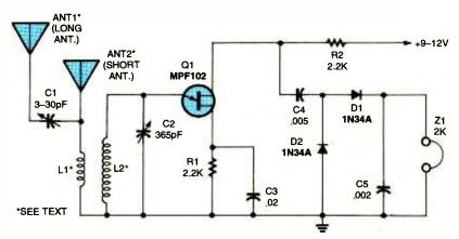
Fig. 2. Unlike the previous circuit, which includes no amplification and uses a single-diode detector—this simple receiver contains a single-stage, tuned-input RF amplifier and a dual diode detector.
