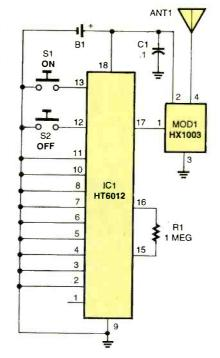
Fig. 1. The Watchdog's transmitter uses a single-chip hybrid module for RF transmissions; no adjustments are needed, and the unit complies with FCC regulations.
