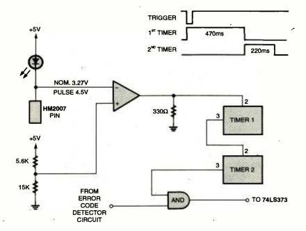
Fig. 2. The interface circuit is designed to monitor the status of the speech-recognition circuit by tapping the cathode voltage of LED1 (in Fig. 1 of last month's column) and feeding it to a voltagecomparator circuit built around an LM741 op-amp.
