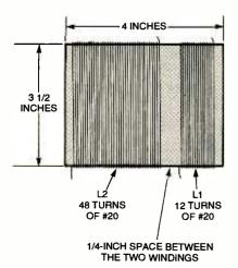
Fig. 3. Details for fabricating the homebrewed coils (L1 and L2)—which are comprised of a total of approximately 60 feet of #20 enameled wire wound on a 4-inch length of 31/2-inch diameter PVC pipe-used in the Fig. 2 circuit is shown here.
