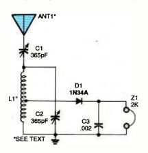
Fig. 1. This simple but functional crystal receiver—comprised of a germanium diode (D1), a hand-wound inductor (L1), and three capacitors (C1–C3)—can tune AM broadcast-band stations transmitting on a frequency ranging between 550 and 1600 kHz.
