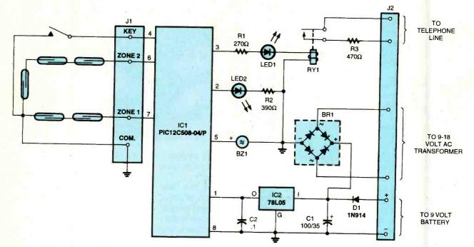
Fig. 1. The Caller-ID Alarm is based on an 8-pin PIC microcontroller. If a switch on either zone is opened, the unit places a telephone call; RYI and R3 mimic a rotary-dial telephone. After the second ring, the system hangs up. That amount of time makes sure that the telephone company's Caller ID information is transmitted to the called number. A battery keeps the system active in case of a 16 power failure—the system only draws 3.5 mA activated.
