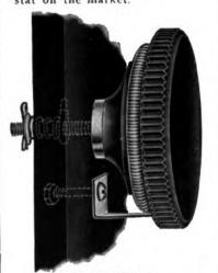
(Actual Size) No. 35 Parkin Panel Type Rheostat (Pat. March 30, 1920) has easily renewed resistance unit mounted on back of moulded Bakelite Knob. Shaft is moulded into knob, cannot come loose. "Off" position provided .3:0 degree rotation insures fine adjustment.
