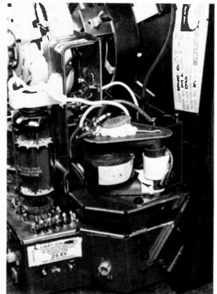
Fig. 28 No high-voltage compartment is needed in the Zenith 4B25C19 chassis; consequently, the high-voltage transformer and the tripler assembly are easily accessible.
