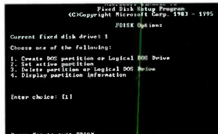
Figure 8. If any partitions already exist on a drive you will need to delete them if you wish to create new ones or resize them.
