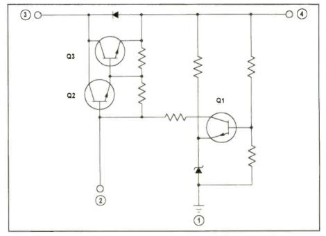
Figure 2. The five terminal regulator comprises error detector Q1, error amp Q2, and seriespass transistor Q3. Pin 5 is unused.
