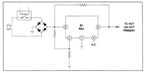
Figure 1. In the conventional design, the 5-terminal regulator is situated downstream of the on/off relay. The regulated output is routed to the HOT via the IHVT primary winding.
