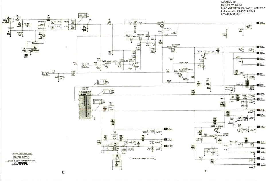
Figure 3. The Magnavox 25P506-00AA uses an unusual circuit configuration to eliminate the need for a power relay. The main B+ regulator goes into a standby mode when the set is off.
