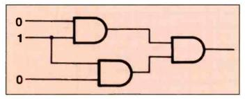
Figure 4. What will be the output of this logic circuit?
