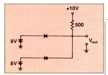
Figure 2. What is the output voltage of this circuit?
