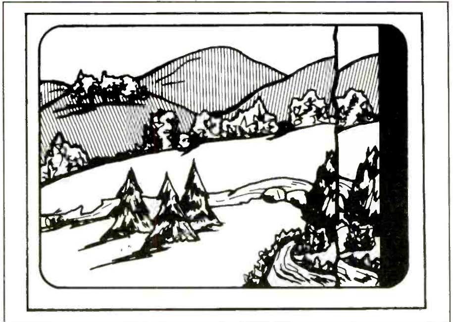
Figure 1. Horizontal foldover in the TV chassis may occur on the right hand side and center of the TV picture or raster.
