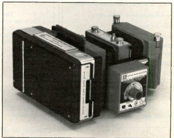
Figure 5. The C-30A camera is designed for loader scopes using the 0.8 cm/div CRT. It has a continuously variable lens arrangement for variable magnification, interchangeable film backs, and it swings away from the scope to allow viewing of the CRT.
