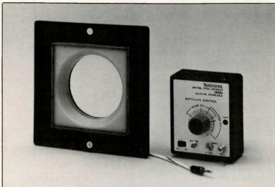
Figure 1. This writing speed enhancement attachment to a CRT fogs the film in the camera. This slight exposure to light increase the maximum sensitivity of the film.
