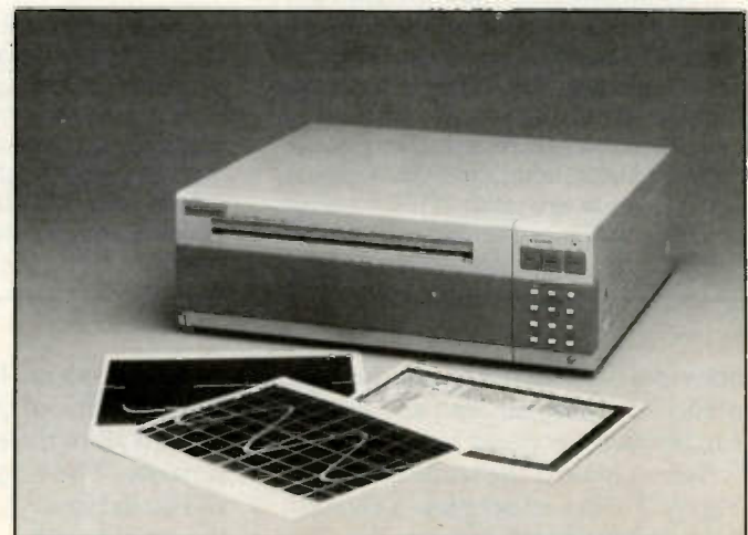
Figure 9. This 9 pin dot-matrix printer can be used to print out a copy of the scope trace captured by a computer-based scope trace recording system.
