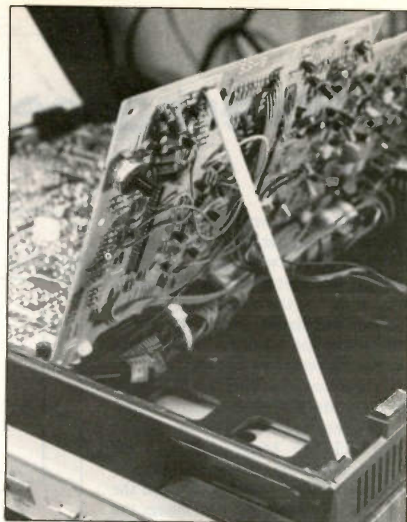
Figure 3. The finished product has a point on one end, a chisel tip on the other end, and a small notch on one side of the chisel tip for snatching wires and the edges of circuit boards.
