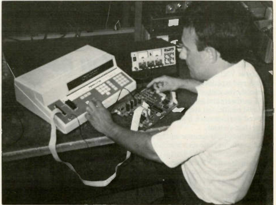
Figure 1. Low-cost functional IC testers can work in-circuit or out-of-circuit. A functional tester is being used here to troubleshoot a microprocessor-based board.
