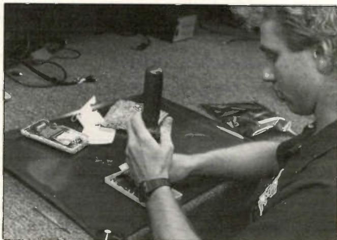
Figure 6. Nintendo video games represent a relatively new class of products that need servicing. Here a technician at Frick refurbishes a Game-Boy unit. This procedure includes replacing certain specified components that tend to wear or fail, and is done at a fixed price.
