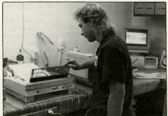
Figure 3. Dot matrix printers such as the one on the service bench are highly reliable, but even they do fail, and require service. In this case, the printer wasn't faulty, but had to be reconfigured via the soft keys on the front to do what the owner wanted it to do.
