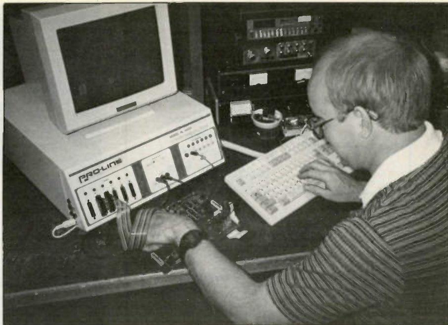
Figure 6. Functional testers can speed troubleshooting of microprocessor-based boards. The board being tested is from gaming machinery.
