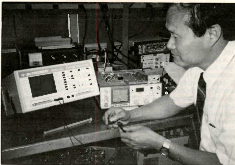
Figure 2. Signature analyzers can be used without known good components for comparison. This is especially true when testing discrete components out-of-circuit
