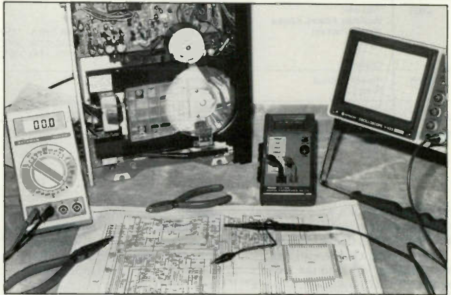
Figure 1. The oscilloscope, digital multimeter, capacitor tester and schematic diagram are required for servicing of CD players.
