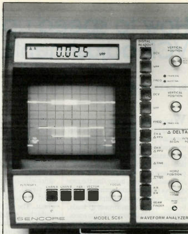
Figure 4. To adjust the record current level, you can measure its value by counting scope graticules. Here the cyan bar is selected by the oscilloscope's delta PPV function. Now all the technician has to do is to adjust the circuit until the digital display shows the correct level.
