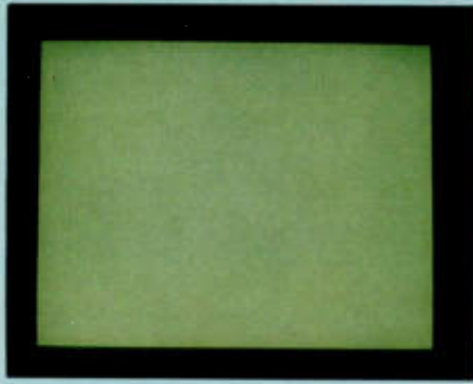
Figure 3. The raster pattern tests color purity.
