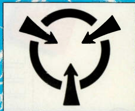
Figure 2. This symbol may be found on military spec. items. It is specified for use by MIL-STD-129J dated September 25, 1984. The military standard specifies what items it must be used on, size, color and wording for products that are to comply with the standard. The symbol is also sometimes used to designate areas where ESD/EOS sensitive materials may be exposed.
