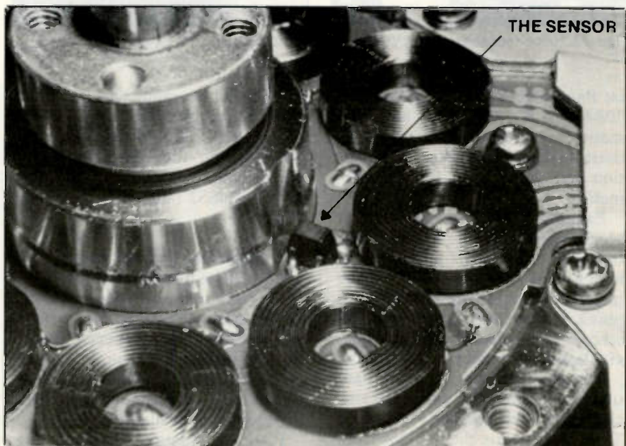
Figure 7. Hall effect sensor in a cylinder head motor.
