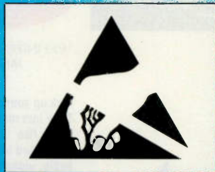
Figure 1. This symbol is related to the standard RS-471 promulgated by the Electronic Industries Association. You will find it on certain items along with wording that describes the hazard. It also is sometimes used to designate areas where ESD sensitive components may be exposed.
