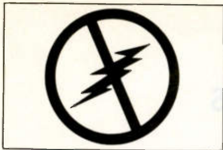
Figure 3. This ESD symbol means "no sparks," and is a symbol meaning that a product or package, such as a container for ICs will not generate static electricity and is therefore safe for use in areas where ESD sensitive components may be exposed.
