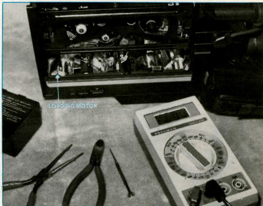
Figure 2. The loading motor is found off to one side in the VHS RCA CPR300 camcorder.
