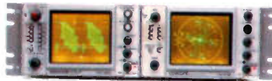
Observing complex video signals is made easy with Kenwood vectorscopes and waveform monitors.
