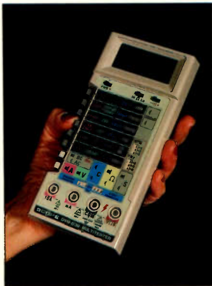
For portable use, the Scope DVM-638 meter usually is held in the left hand, thus permitting thumb operation of the edge-mounted switches.
