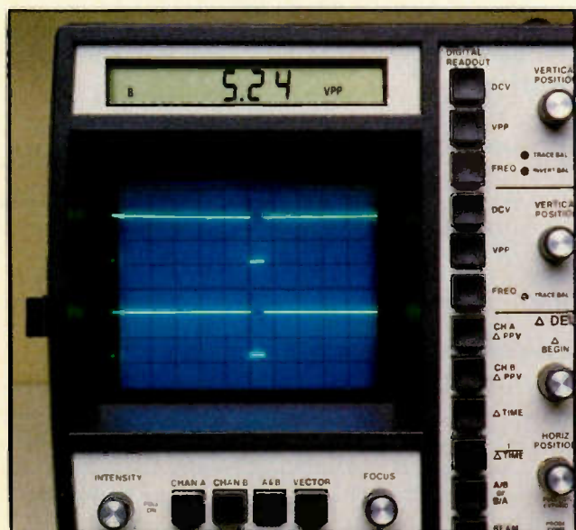
Figure 6. When troubleshooting keyboard problems, use the dual-trace function to compare the timing of the scanning pulse and the data pulse. The keyboard schematic then tells you which switch contact is closed.
