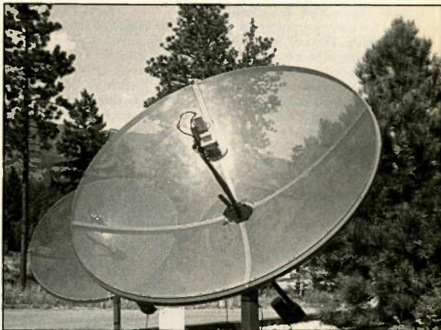
If the feed-assembly shadow falls on the center of the parabolic reflector, the solar energy collected by the reflector is concentrated at the focal point, which is where the feed assembly is located.
