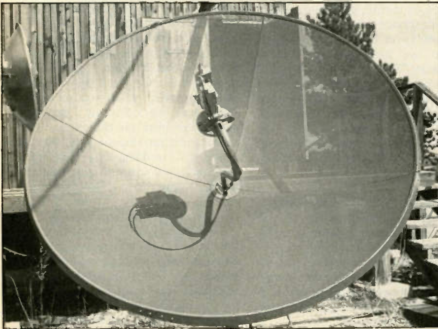
The feed-assembly shadow indicates that the sun is east of the satellite to which the dish is pointed. As time of day advances, the shadow will move toward the reflector center.
