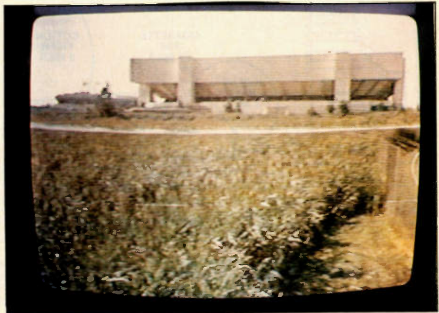
Figure 1. Most tape dropouts are not visible in actual use because a delay line in the VCR uses the previous horizontal scan line to fill in lost information. However, a severe dropout, such as the one shown here, will be visible.
