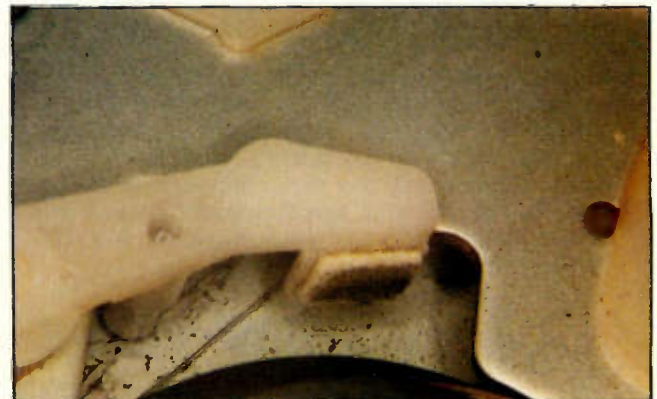
Figure 4. Dirt on the sub-brake T pressure pad.
