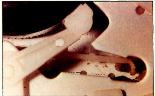
Figure 2. A close-up of the sub-brake T in stop mode.
