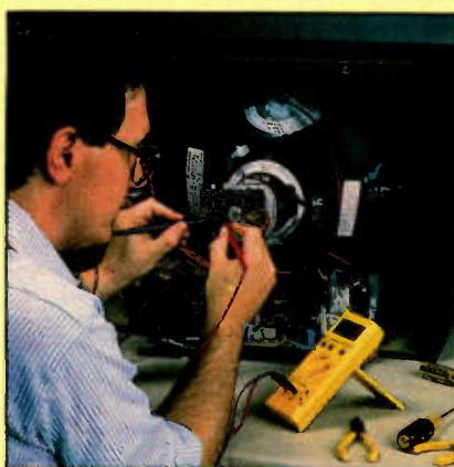
Figure 2. Some of the newer features such as autoranging and audible readout make it easier to concentrate on the work, not the tool.
