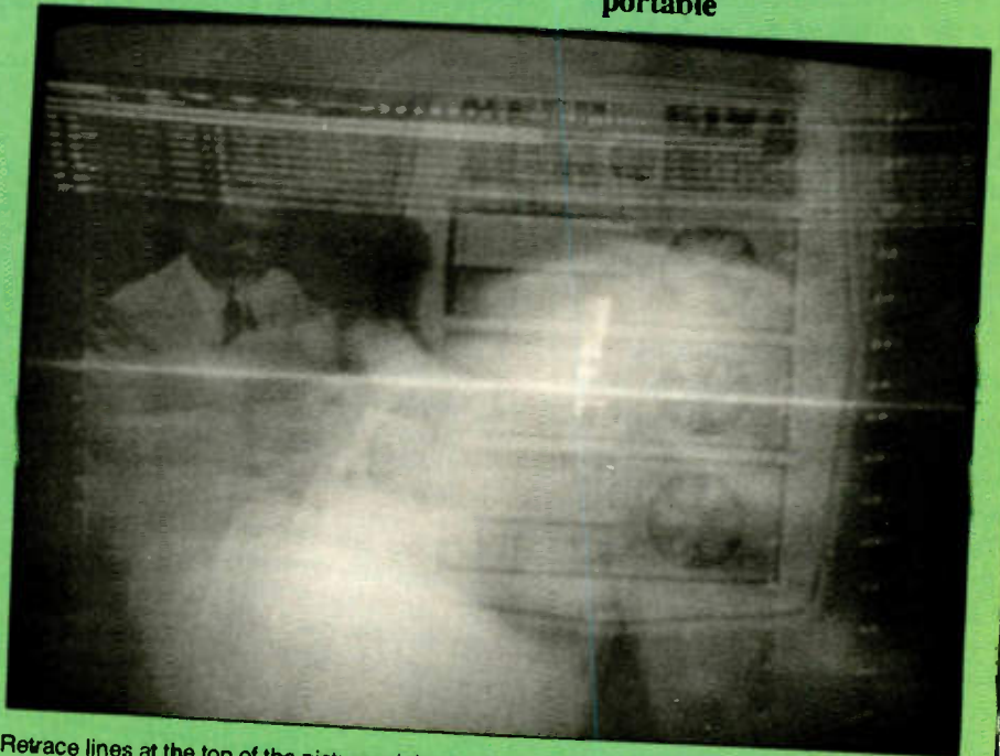
Retrace lines at the top of the picture might result from defective components in the luminance, picture tube or vertical circuits.
