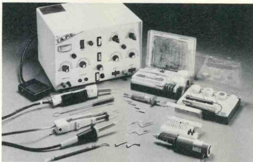
A repair and rework center, such as this one offered by A.P.E. provides facilities to completely repair all printed circuit board types: conventional, S-M, hybrid.
