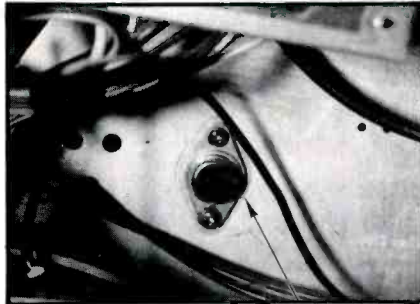
Figure 2. The second regulation is accomplished by Q801, located on the metal chassis (using the metal as a heat radiator or sink). A defective Q801 is common. Accurate testing of Q801 might require its removal from the chassis.
