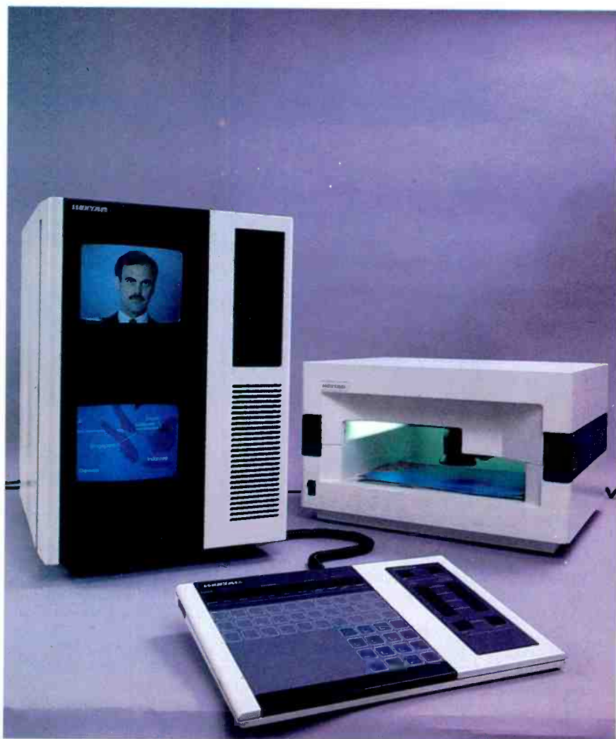
The newly introduced Personal Videoconferencing Station (PVS) designed for business and government applications offers the following features: dual memory still-store system; 6-color electronics blackboard; alphanumeric character generator; copy stand and variable audio system.
