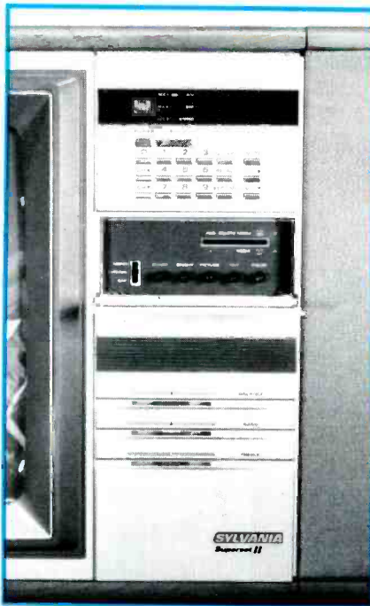
Figure 2. Push-buttons and other controls are arranged in four areas of the Sylvania front panel: the remote sensor and indicator lights at the top; push-buttons for many functions are below; TV controls and other switches are under a hinged door near the center; and balance, bass and treble controls are near the bottom.
