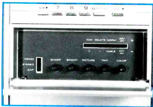
Figure 5. The seldom-used TV controls and some very important switches are located under the hinged door (seen at the bottom, a bit out of focus). If the AV switch is pushed in to the on position, the screen will show a blank raster and there will be no sound unless external audio and video are connected to the jack panel. If the mono-stereo switch is moved accidentally to the SAP position during normal TV reception, the sound will be eliminated. Details are given in the text.
