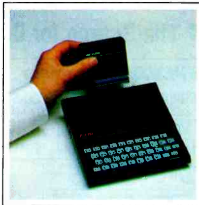
A plug-in RAM pack adds 16kBytes of random access memory to the ZX-81.
