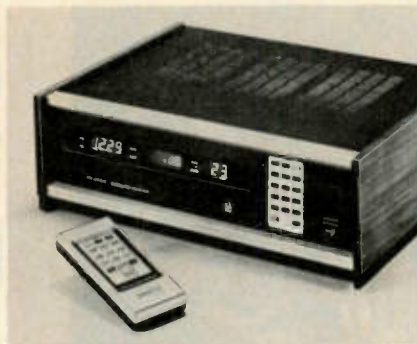
Figure 3 The Heathkit Satellite Receiver is an attractive unit that can be placed on top of most TV receivers. Output of the Satellite Receiver goes to the antenna terminals of a standard TV receiver. The unit is larger than some videocassette tape recorders, and features many new technical conveniences such as direct-access electronic tuning with remote control.
