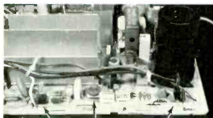
Figure 5 This backside view of the M10 module shows ICX3301 (left arrow), factory-adjusted control RX3312 (center arrow), and Q3301 forward horizontal driver (arrow at right).
