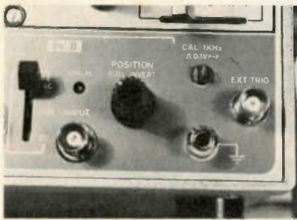
Figure 5 A polarity-inversion function has been added to the channel-B positioning control. Also shown are the calibration-waveform output, the instrument ground post and the external triggering input plug.
