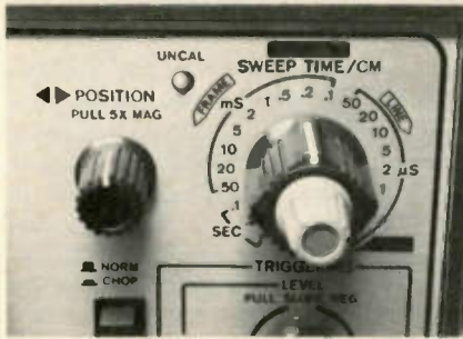
Figure 11 This is a closeup of the sweep-time/cm and 5X magnification controls mentioned briefly in Figure 7. The shortest sweep time is 0.1\mu\text{S} , which divided by the 5X expansion provides the equivalent of 0.02\text{ S/cm} (or 20\text{ns/cm} ) sweep.
