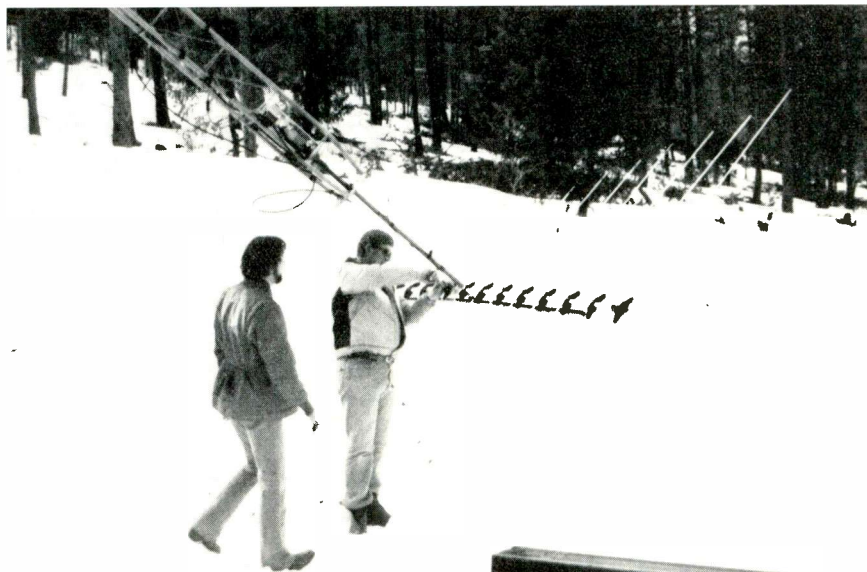
Before making polar-plot and gain measurements at the Winegard Research Laboratory in Evergreen, CO, an engineer-technician team installed an antenna on a rotating mast that is the top of a tilting tower. The tower was pulled upright before the tests.
