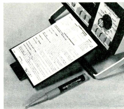
Figure 3 A TP222 probe that slips over the regular test probe allows direct-reading dc voltage measurements up to 9.999kV when the DCV-10KV PROBE function is selected. A plastic card with condensed instructions for operating model DVM-56 can be slid out from beneath the DMM when needed.
