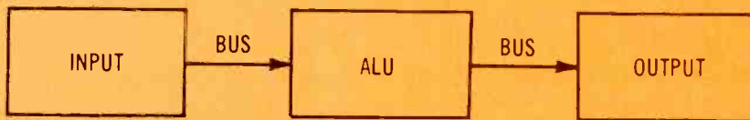
Figure 1 The Arithmetic-Logic Unit (ALU) of a microprocessor with suitable encoders and decoders can perform many mathematical calculations and logic functions. However, the human operator must manually control each step.
