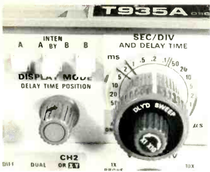
Figure 16 The seconds/division switch assembly of the T935 Tektronix has three functions. The position of the large knob determines the primary sweep time. When it is pulled out and turned to the right, the sweep time of the delayed sweep is selected. The small knob at the outside is a variable width control with calibrated X1 and X10 positions at the stops. Also, the three buttons and knob at the left are used with the delayed sweep. This delayed sweep can greatly expand small areas of a waveform.
