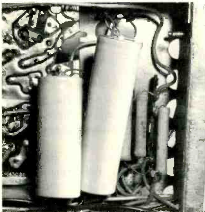
Figure 2 Paralleling new capacitors across the old ones if not recommended. Failure of a second section often follows the original failure. These capacitors are too near the hot resistors, and their size further restricts the air flow.
