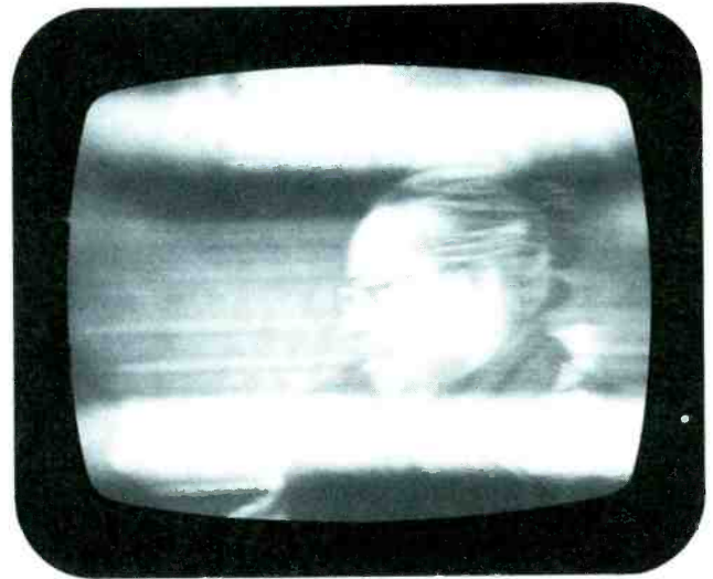
6—Two light or dark round-edged horizontal bars floating up the picture are proof of 120-Hz hum. The frequency indicates a filtering defect in a full-wave power supply. Often these are called "hum bars".
