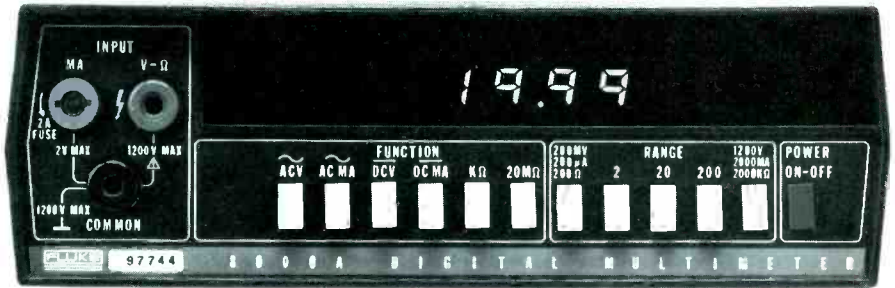
Resolution is 100 microvolts, 100 nanoamps and 100 milliohms
