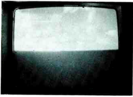
Fig. 7 An open in either of the complementary-symmetry vertical output transistors can limit the deflection and move it to either the top or bottom, depending on which transistor is bad.
