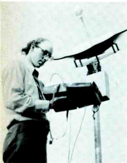
An engineer adjusts the orientation of a parabolic "dish" satellite-receiving antenna while watching a signal-strength meter. Experimental equipment manufactured by RF Communications, Inc.
