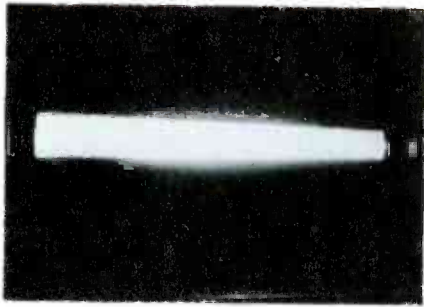
Fig. 6 At first glance, this might seem to be a case of insufficient height. However, the left edge is taller than the right, so it is a trapezoidal picture. One vertical-yoke coil was open, and a higher-than-usual load resistor supplied only a small amount of deflection.
