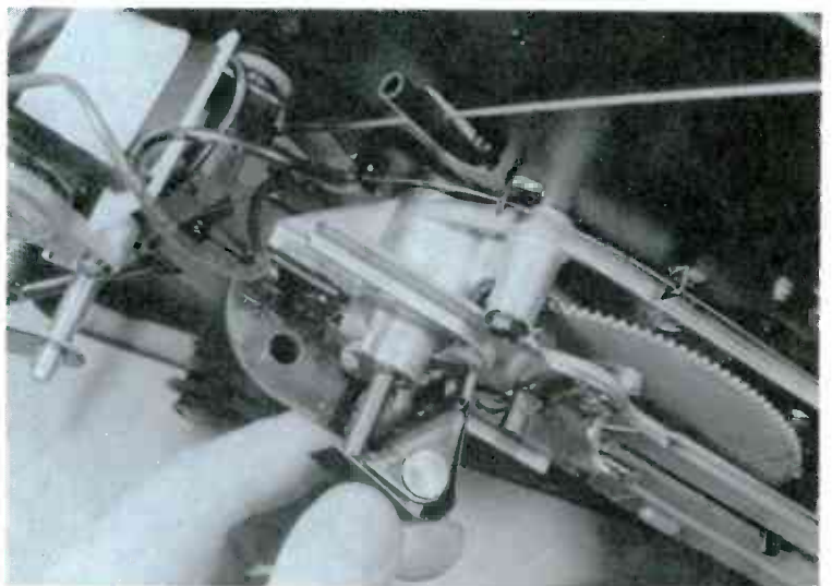
Step 9 The spindle in most record changers can't easily be removed as it can from automatic turntables, for it has more to do with record dropping. The cycling slide, as it reaches almost the half-cycle position, encounters a rocker-type pawl. That lifts the center rod of the spindle, operating the pushoff tab and dropping the record.
