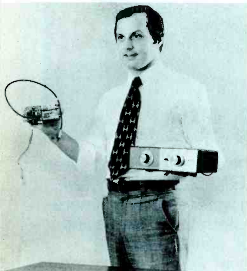
John Meelan is holding in his right hand the 24-channel solid-state RCA cable tuner. It does the same job as the larger unit held in his other hand, a converter that is placed on top of the conventional TV receiver.
